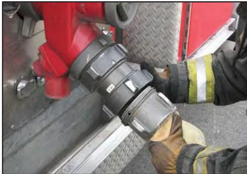
LDH connected to the main side intake using a 4" double female.
