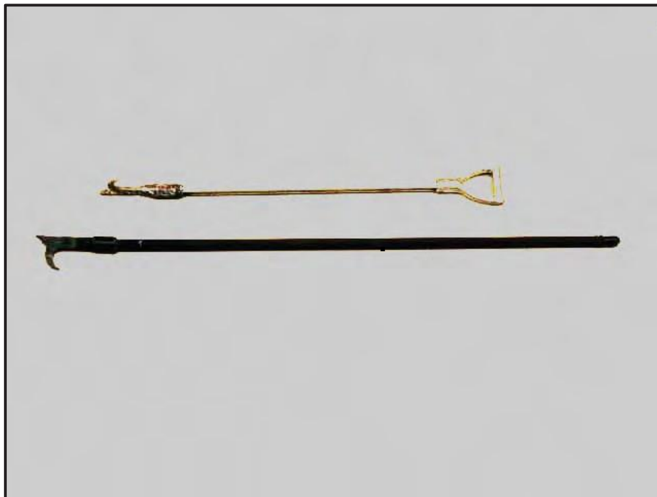
D-Handle and Straight Handle Pike Poles
