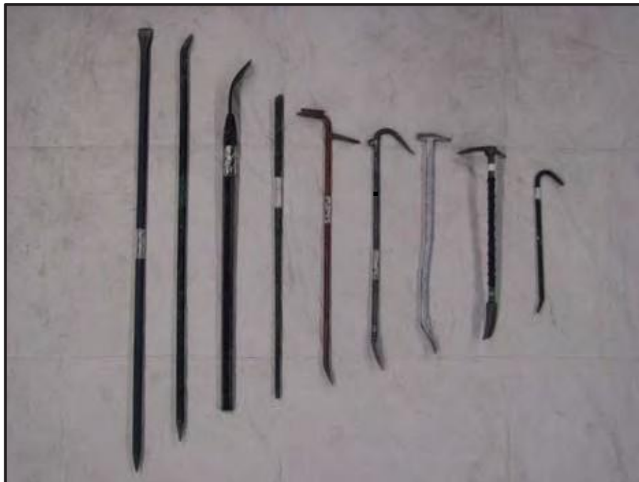
Left to Right: Heavy Duty Bar, Medium Duty Bar, Burke Bar, Light Duty Bar, Extrication Bar, Lock Breaker, Trumpet Bar, Haligan, Wrecking Bar
