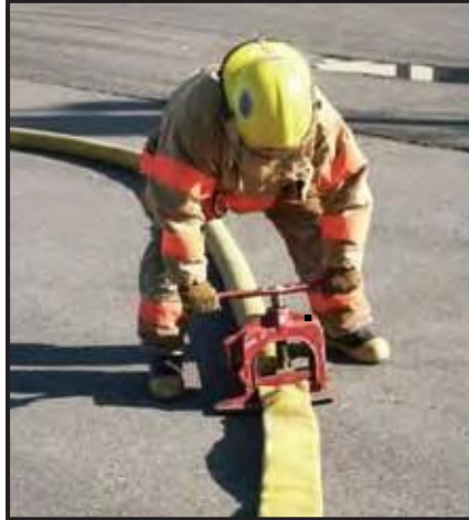
Face the direction of the flow when opening the hose clamp.
