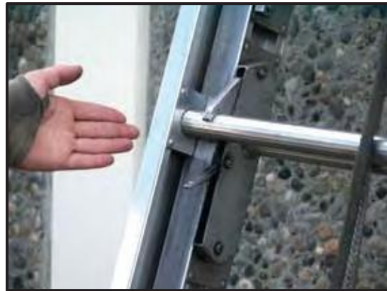
Correctly locked dog
