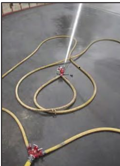
Finished Monitor Manifold.
