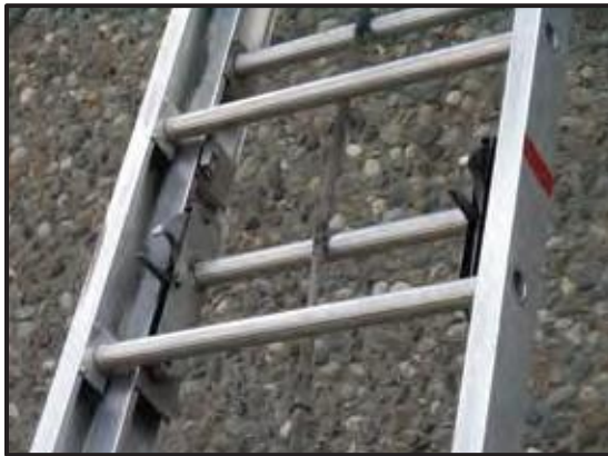
Dogs between rungs during extension of the fly
