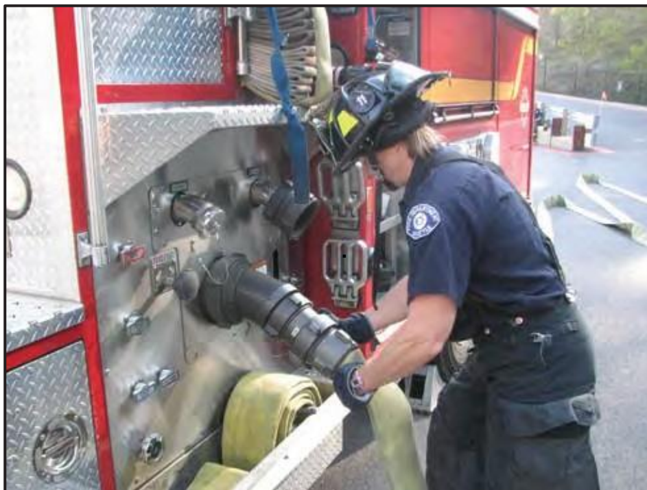
Making the connection to the intake with a 4" double female coupling.
