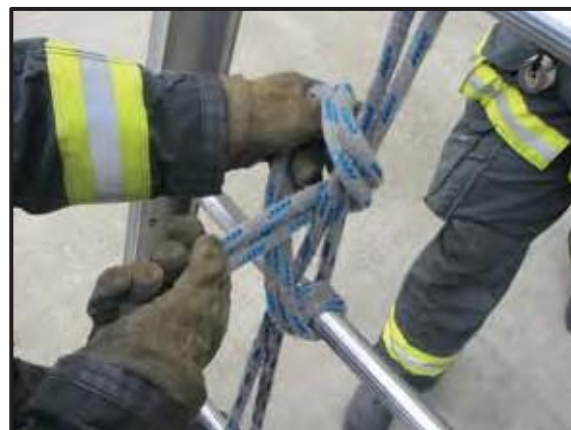
Tie a half-hitch around the halyard above rung 3
