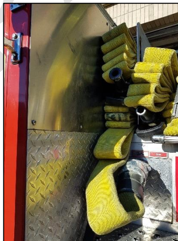
2 1/2" Pre-connect "Blitz" Line (Slot Load)
