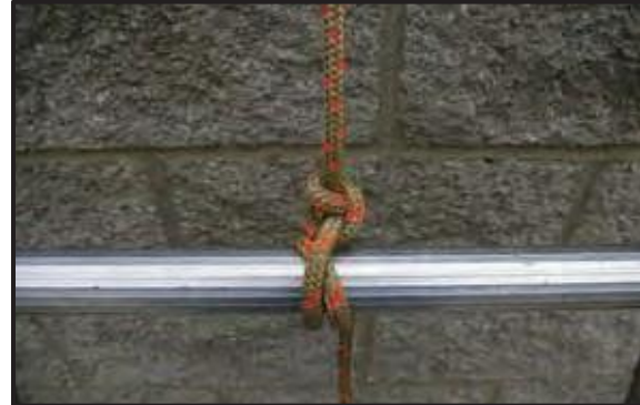
Tie two half-hitches above rung 2 onto the rope between the two rungs
