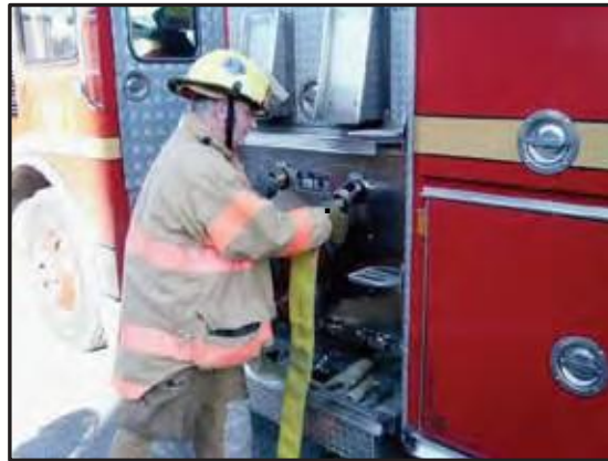
Making the connection to the discharge port.
