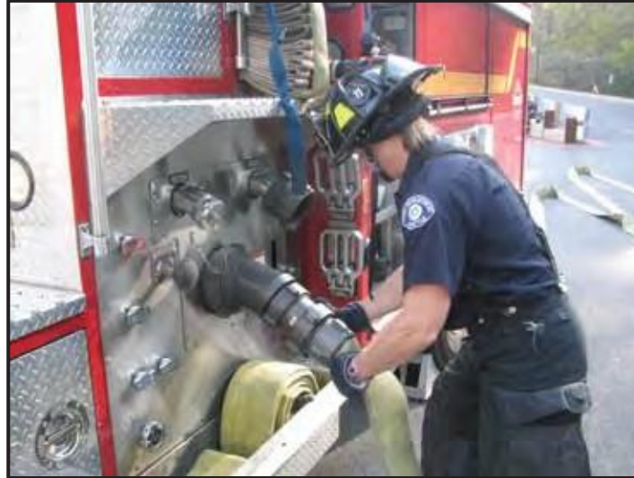
Connect the LDH to the main side intake.
