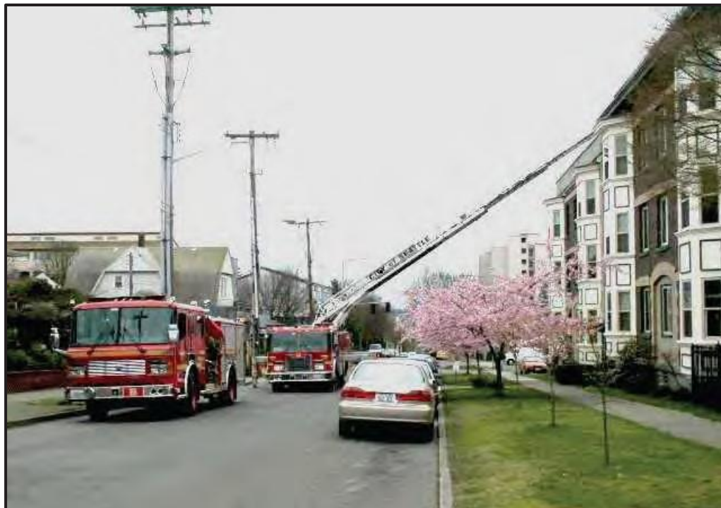
The engine company positioned for proper ladder company access.
