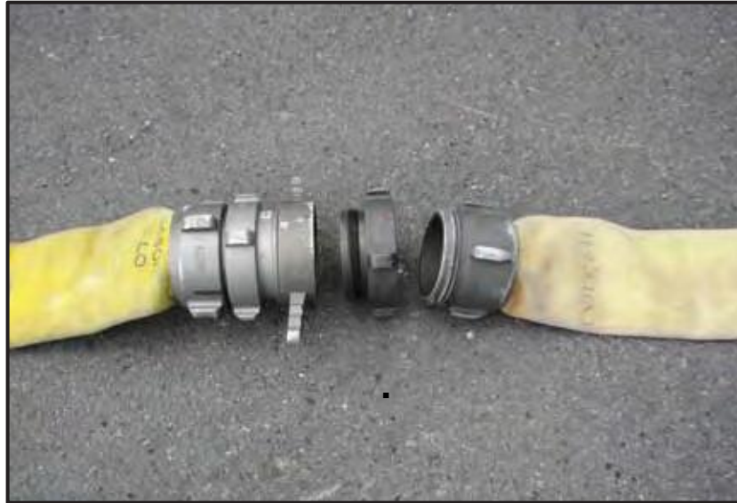
Soft suction extended with a section of LDH using the soft suction adaptor (red marking).
